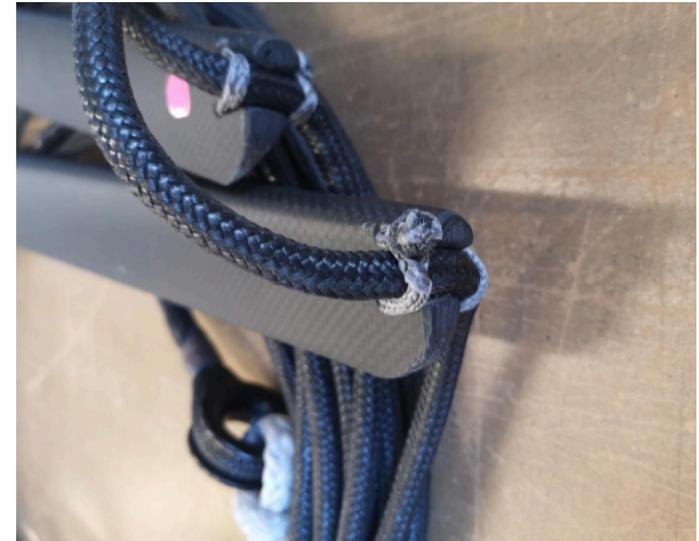
Attach shrouds to mast in their respective positions. Starboard side and port side shrouds are marked with blue and red duct tape on the top fittings, respectively.
