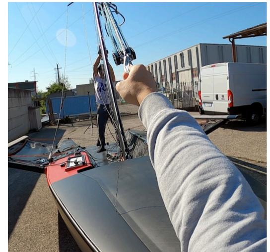
Lift the mast up pivoting about the foot with one person pulling from the forestay tensioner line, and one inside the boat pulling up the mast ( be aware that with the weight of the people in the back of the boat it will topple so you will need something under the back or someone on the bow to avoid it).
