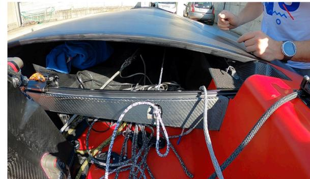
Now attach the other shrouds to the loop, the D2 on the further one and D1 in the middle one and take a bit of tension and attach the forestay loop to the ring to continue working on the boat.
