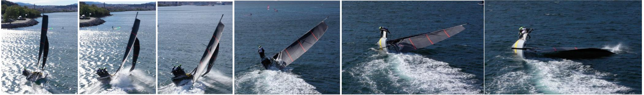
The racks are also slowing down the capsizing therefore usually the crew has some time to move up to the boat's side without going into the water.
