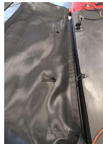
Pass the gennaker sheet block's soft shackle through the cut in the net.
