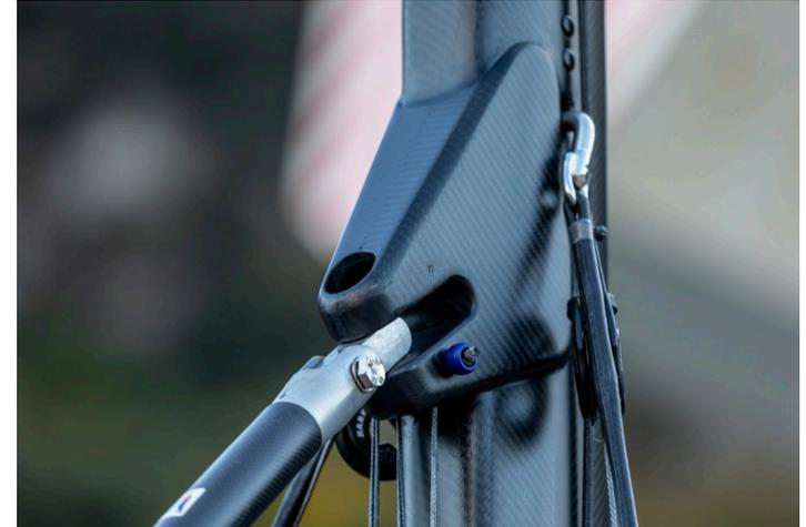
Bolt the boom fork to the boom gooseneck.
