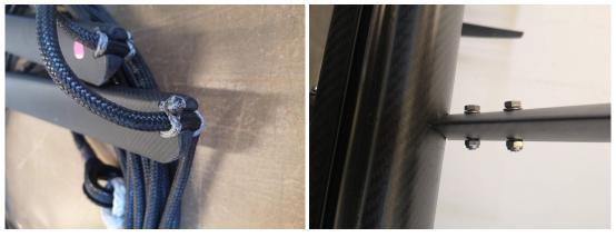
Attach shrouds to mast in their respective positions. Starboard side and port side shrouds are marked with blue and red duct tape on the top fittings, respectively
