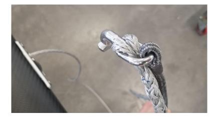
• Attach forestay making sure to pass it through the deflector ring. The jib halyard must
