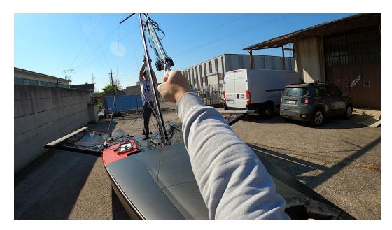
Pass the tensioner's soft loop around the bowsprit and pull the bowsprit out for safety.
