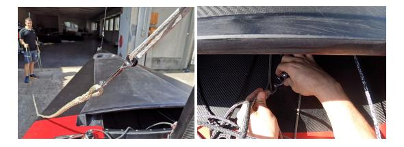
Lift the mast up pivoting about the foot with one person pulling from the forestay tensioner line
