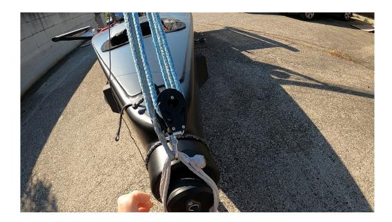
• Pull the halyard purchase almost completely and make a safety knot aft of the cleat.
