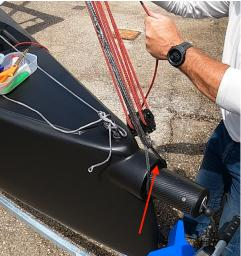
2. Check the mast is symmetrical port-starboard by measuring the distance between the hoisted halyard and the boat sides in a position of your choice (e.g. V1 shroud attachment point on deck).
