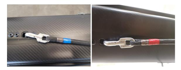
Before attaching the forestay, cow-hitch the spliced end of the jib halyard to the forestay top fitting. The jib halyard running outside of the mast is 2:1
